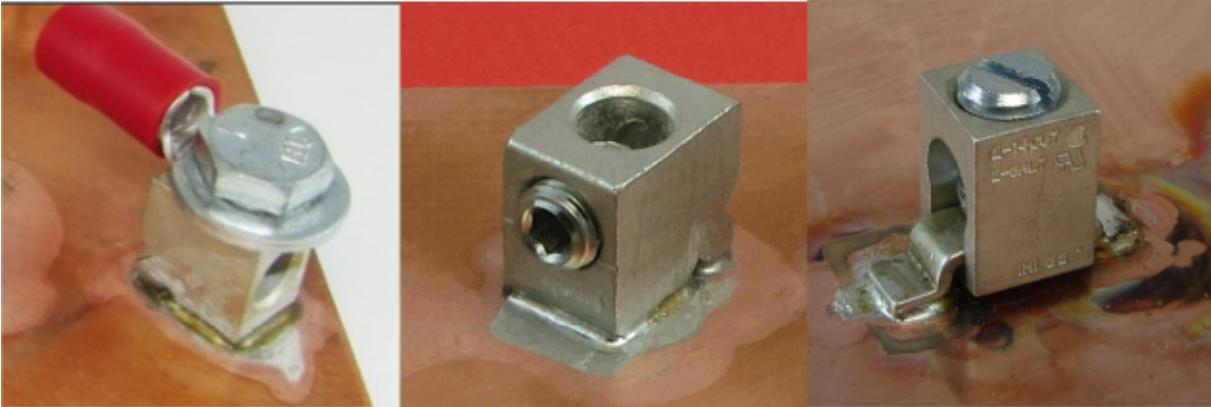
The typical edge fillet on the IHI Solderable terminal in SMT mode is about .025" rad. (varies with amount of solder/paste used) so we suggest that the copper pad showing through the masking would be .050" total wider than the physical contact footprint to accommodate the .025" all around.
